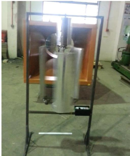
Figure 7: Mix Wind Turbine full assembly during experimental works
