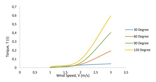
Figure 11: Graph of Torque,  $\tau$  Against Wind Speed, V Produce for Savonius Rotor
