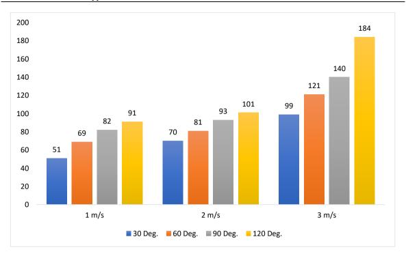
Figure 10: Savonius RPM With Load Based On Blades Curve
