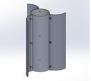
Figure 3: Three-Dimensional View of Savonius Wind Turbine
