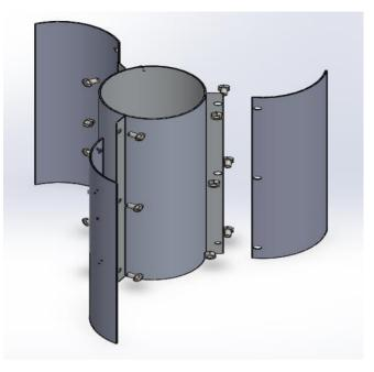
Figure 4: Exploded View of Savonius Wind Turbine
