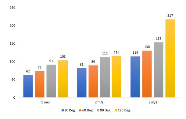
Figure 9: Savonius RPM Without Load Based on Blades Curve
