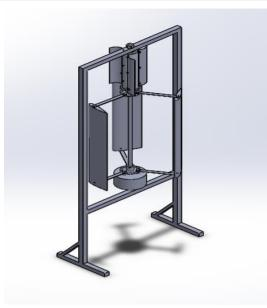
Figure 6: Three-Dimensional Drawing of Mix Wind Turbine
