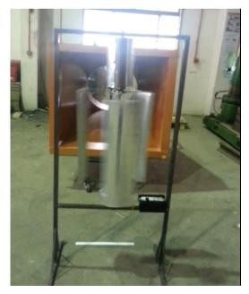
Figure 7: Mix Wind Turbine full assembly during experimental works
