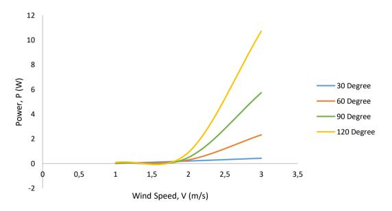
Figure 13: Graph of Power, P Against Wind Speed, V for Savonius Rotor
