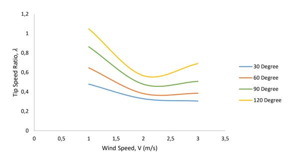
Figure 12: Graph of Tip Speed Ratio,  $\lambda$  Against Wind Speed, V for Savonius Rotor
