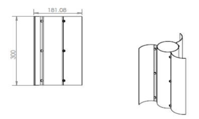
Figure 5: Two-Dimensional Drawing of Savonius Wind Turbine
