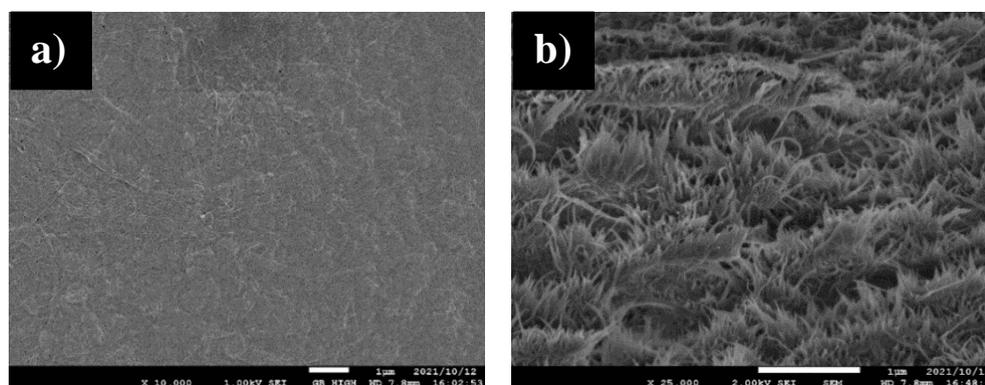
Figure 2 : SEM images of the surface (a) and cross section (b) of the CNF sheet.
