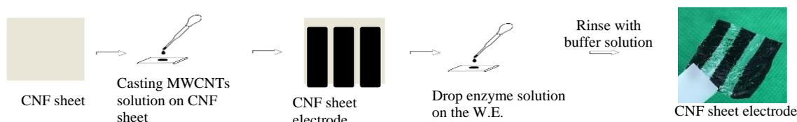
Figure 1 : Scheme of CNF electrode preparation.
