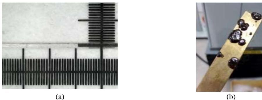
Figure 1: The difference between (a) successfully extruded PET fibers and (b) degraded PET melts at 250°C.
