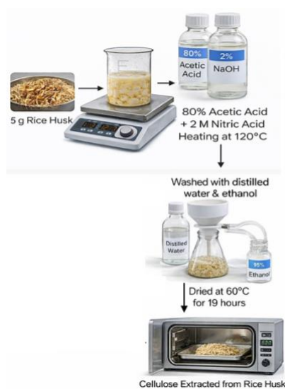
Figure 2. The cellulose extraction process from rice husk
