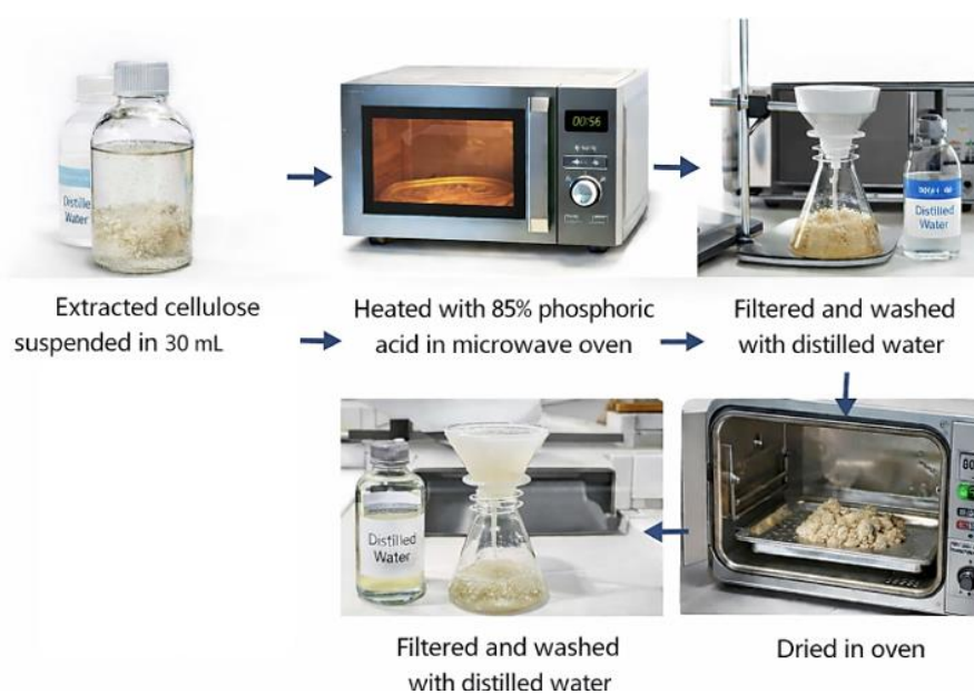
Figure 4. Bio-based absorbent hydrogel Synthesis Process
