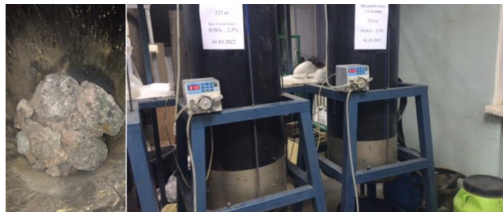
Figure 2: Percolators for heap leaching simulating experiments
