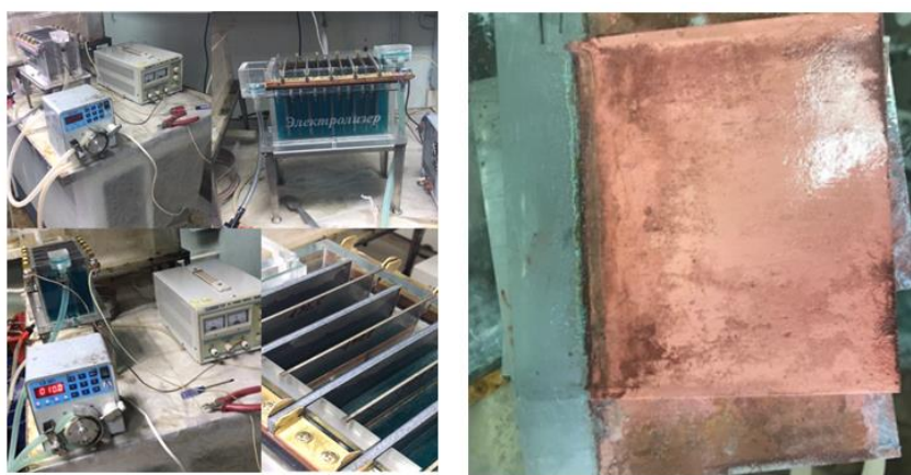
Figure 9: Copper electrowinning process from a saturated electrolyte
