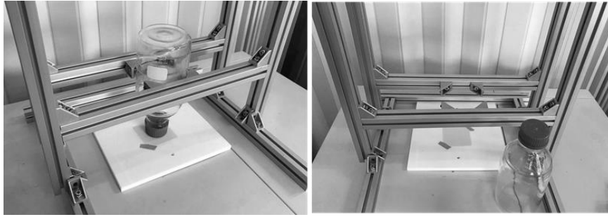
Figure 1: Measurement system for load capacity measurements
