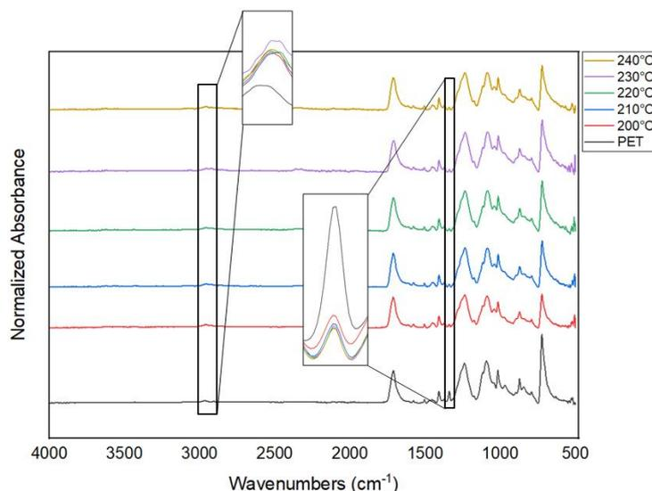
Figure 3: FTIR spectra of recycled PET fibers at various processing temperatures.
