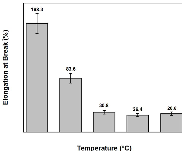
Figure 6: Elongation at break of the recycled PET fibers at various processing temperatures.
