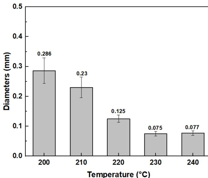
Figure 2: The diameters of recycled PET fibers at various processing temperatures.
