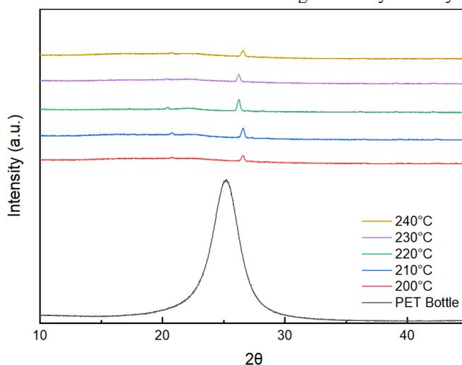
Figure 4: Diffractometer spectra of recycled PET fibers at various processing temperatures.
