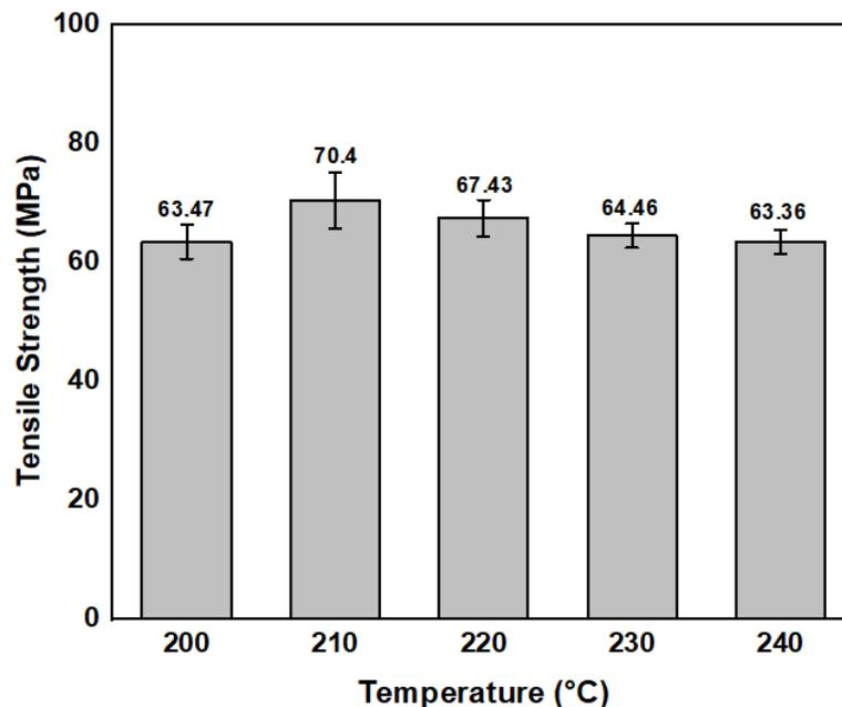
Figure 5: Tensile strength of recycled PET fibers at various processing temperatures.
