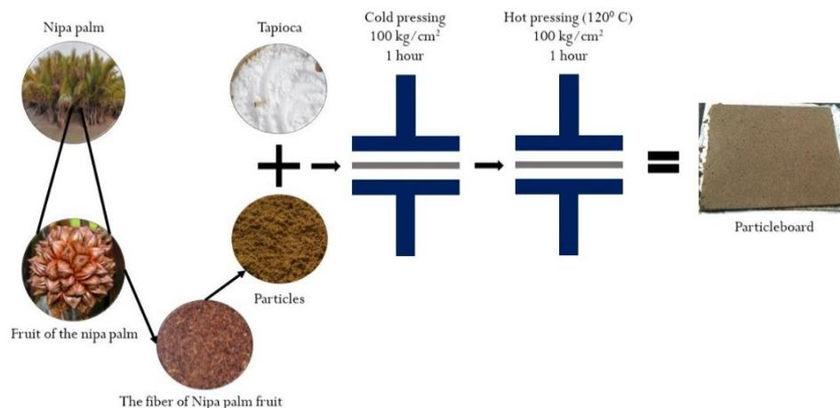
Figure 1: The fabrication of Nipah-based particle board
