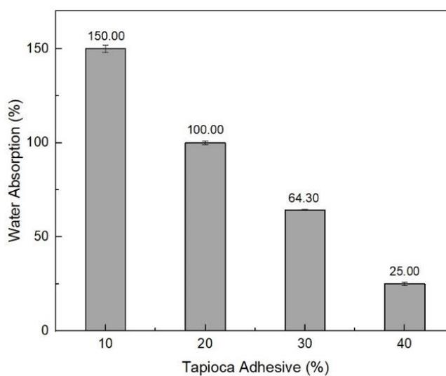
Figure 4: The water absorption percentage of Nipah-based particle board
