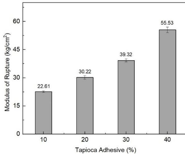
Figure 6: Modulus of Rupture of Nipah-based particleboards at various tapioca concentrations
