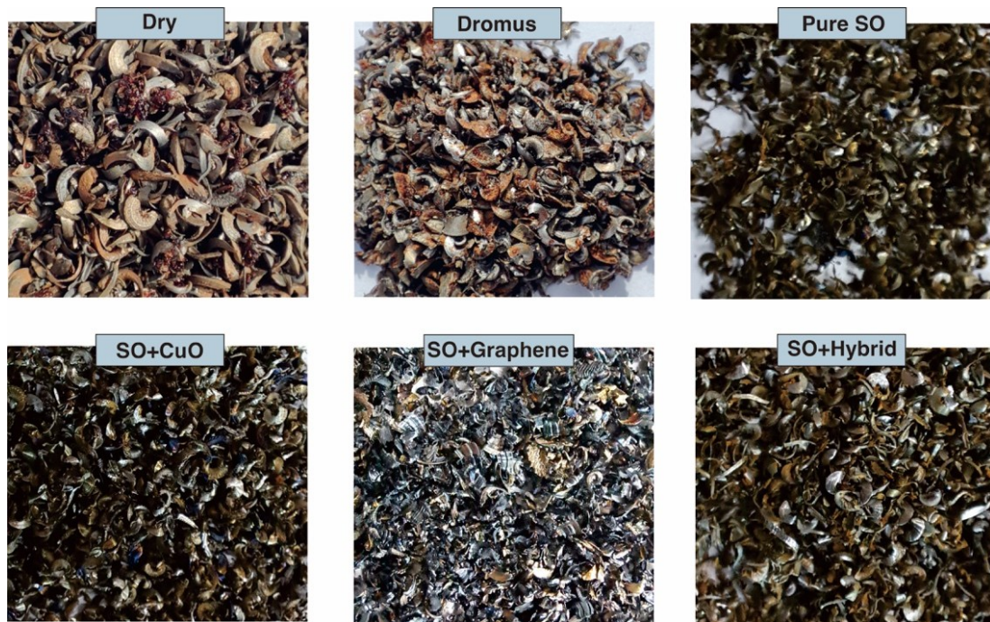
Figure 18. Chip color after application of cutting fluid samples in CNC milling
