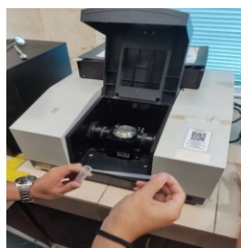
Figure 6. FTIR analysis of the oil samples using the Shimadzu IRAffinity-1 spectrophotometer
