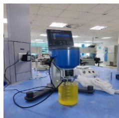
Figure 5. Viscosity measurement of the oil samples using the IKA ROTAVISC lo-vi rotational viscometer
