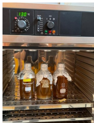
Figure 2. POME-Nanofluid samples undergoing accelerated ageing in a thermal oven
