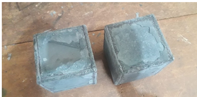
Figure 1. Carburizing media prepared according to the specified material ratios; charcoal and shellfish shell powder powder–charcoal mixture in the carburizing boxes
